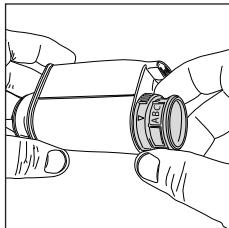
Remove the INTENZA+ water filter from water. Set the machine according to the measured water hardness (see the "Measuring water hardness" chapter) and the letters found on the filter base:
