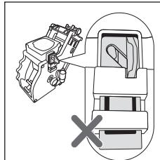
If the hook is still in a lower position, this means that it has not been correctly positioned.
