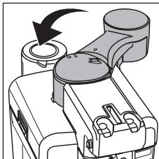
**Warning:** the carafe dispensing spout is to be tightly closed and aligned with the handle to prevent water/steam splashing or puffing.
