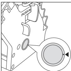
Make sure that the lever is in contact with the base of the brew group.
